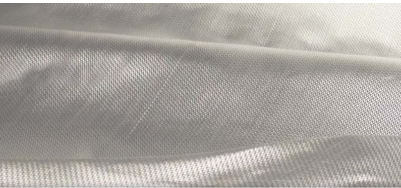
Tyfo® WEB system Bi-directional glass composite ( 0^\circ/90^\circ )
