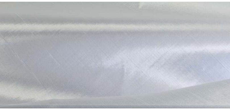
Tyfo® BC system Bi-directional glass composite ( \pm 45^\circ )
